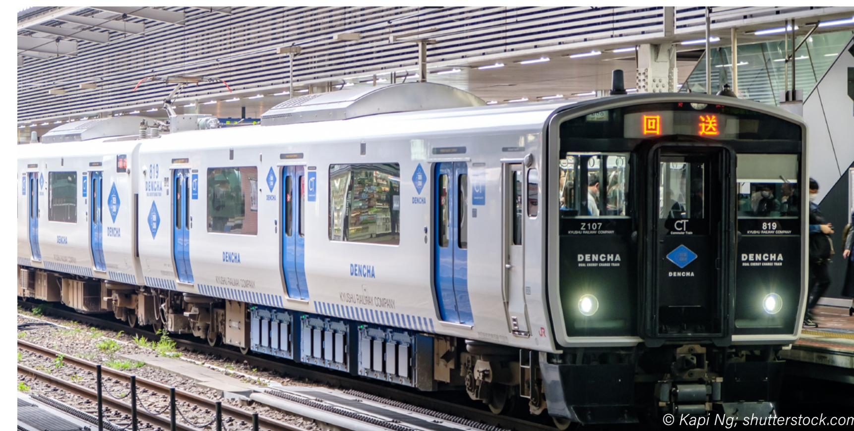
JR Kyushu BEC819 series commuter train. Battery-powered train, that can be operated on a non-electrified line; Fukuoka, Japan
