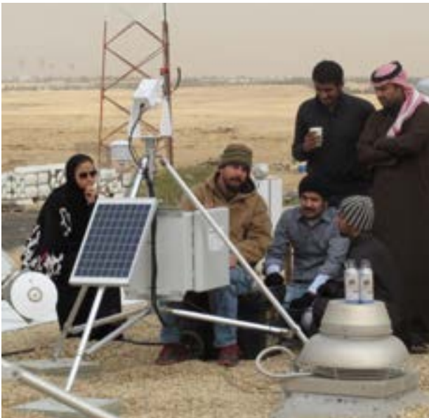
Engineers from NREL and K.A.CARE installing a rotating shadowband radiometer near Riyadh.
